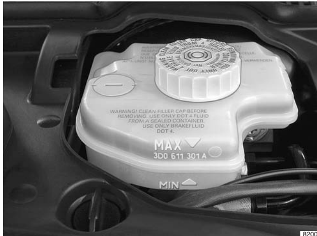
Fig. I-7 Brake fluid reservoir
