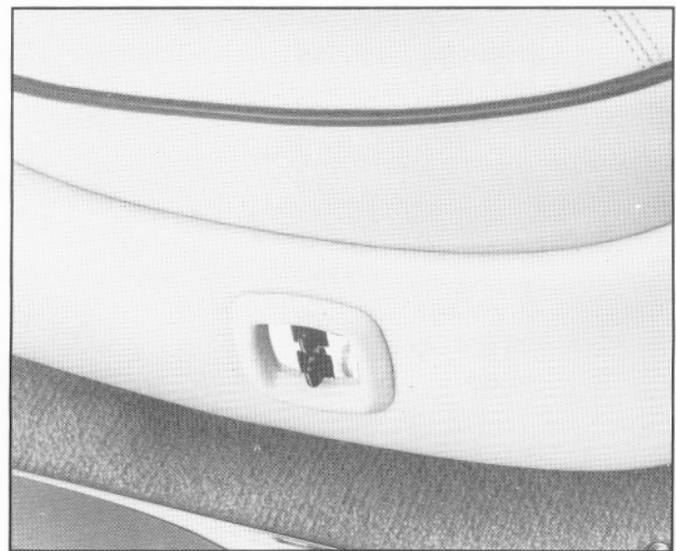
Fig. 18 Front seat lumbar support switches
