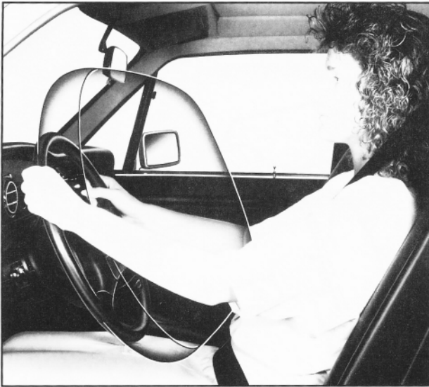
Fig. 20 Driver's airbag passive restraint system
