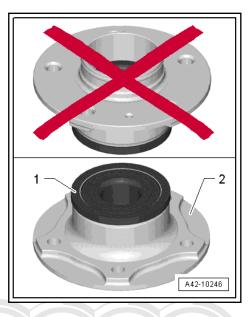
Always set the wheel bearing unit down on the wheel hub -2-.
