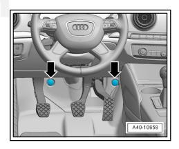
Remove the screw -1- for the universal joint -2- and then remove the universal joint in direction of -arrow-.
