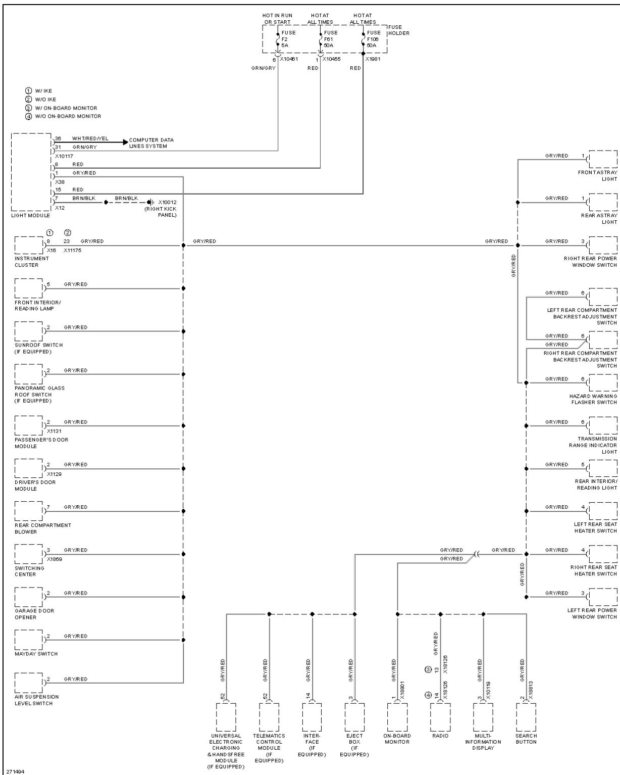
**Fig. 71: Instrument Illumination Circuit**
