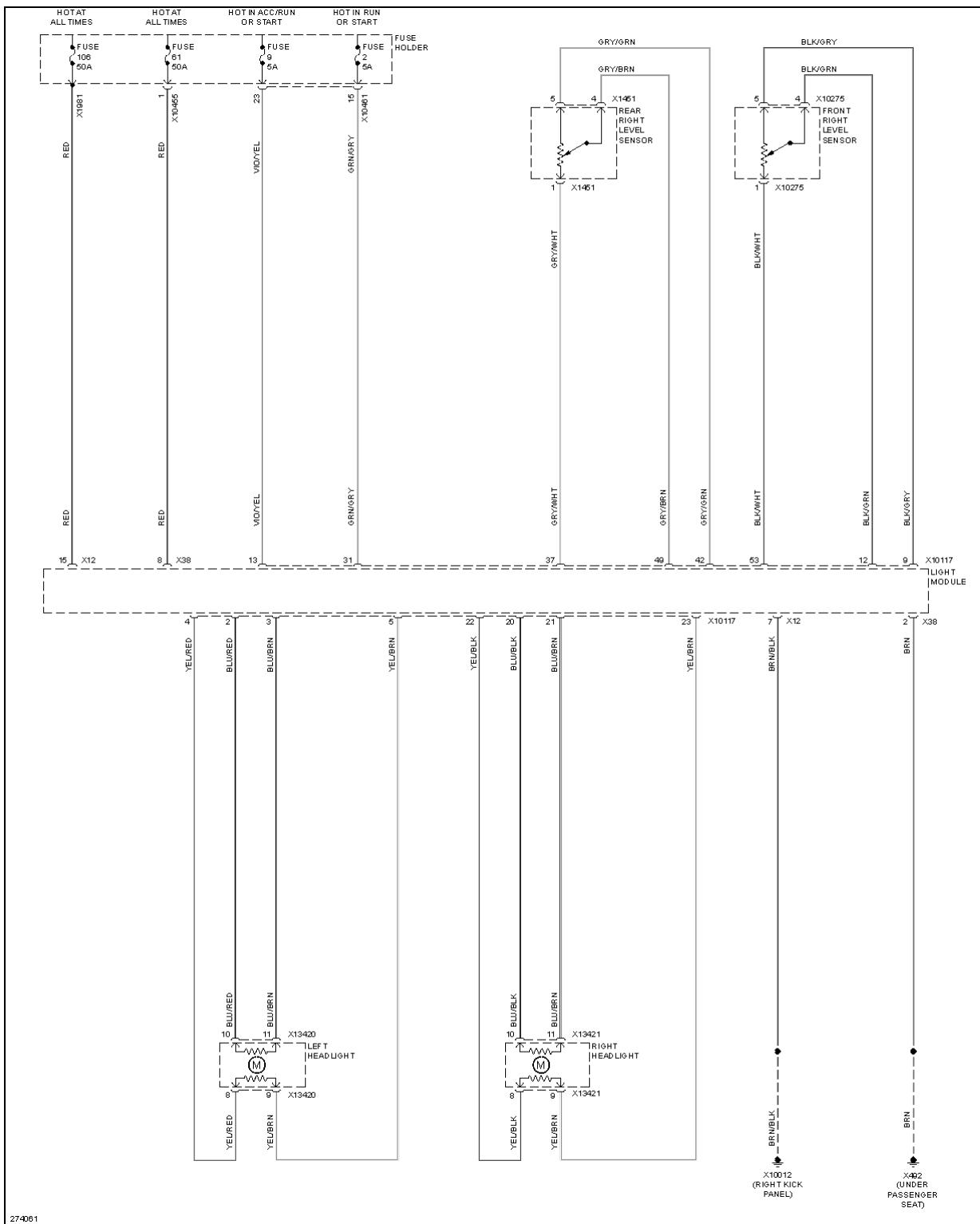
**Fig. 60: Headlamps Leveling Circuit**
