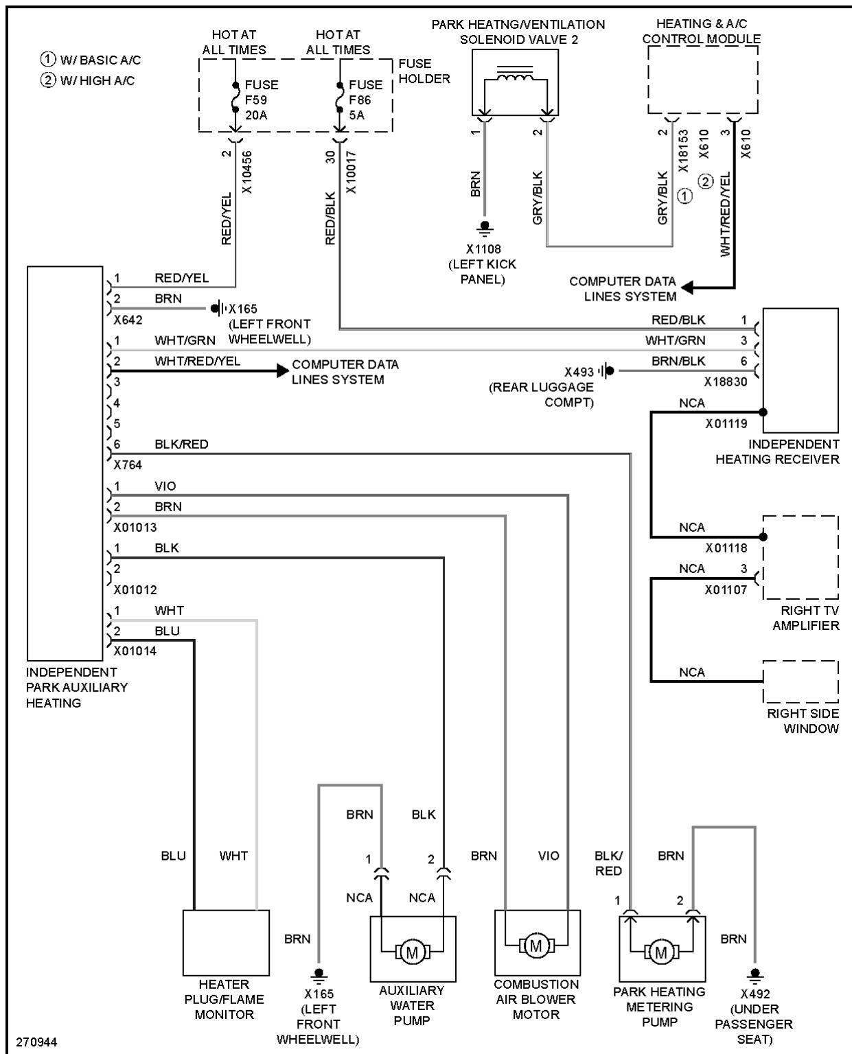
**Fig. 7: Independent Heating Circuit**
