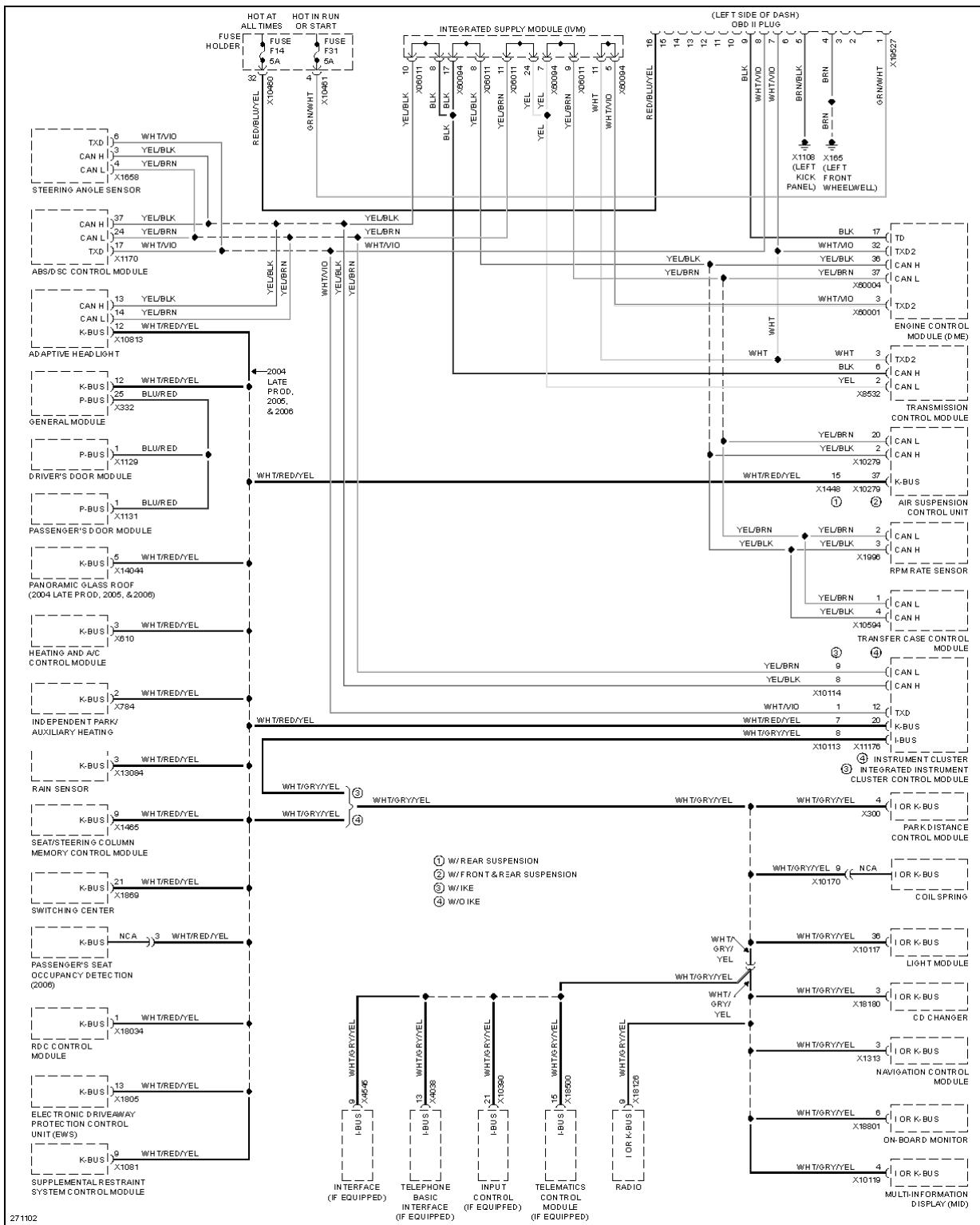
**Fig. 18: 4.8L, Computer Data Lines Circuit**
