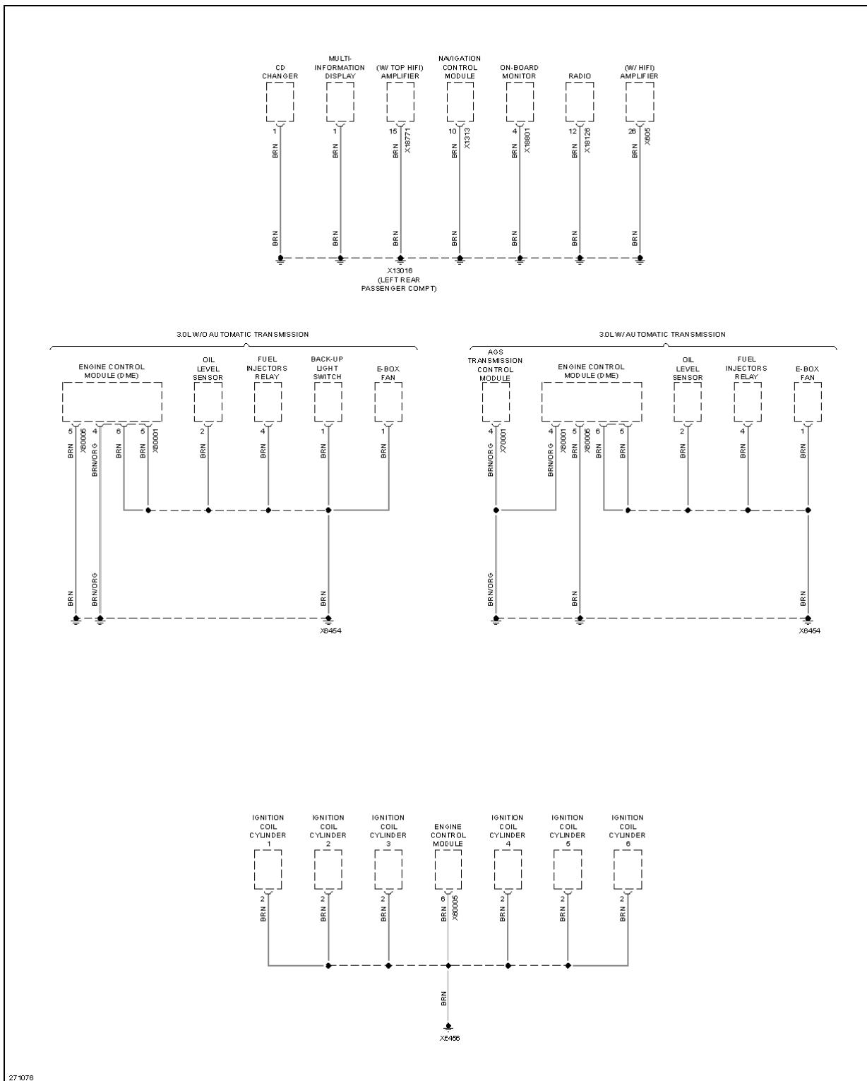
**Fig. 52: Ground Distribution Circuit (5 of 5)**
