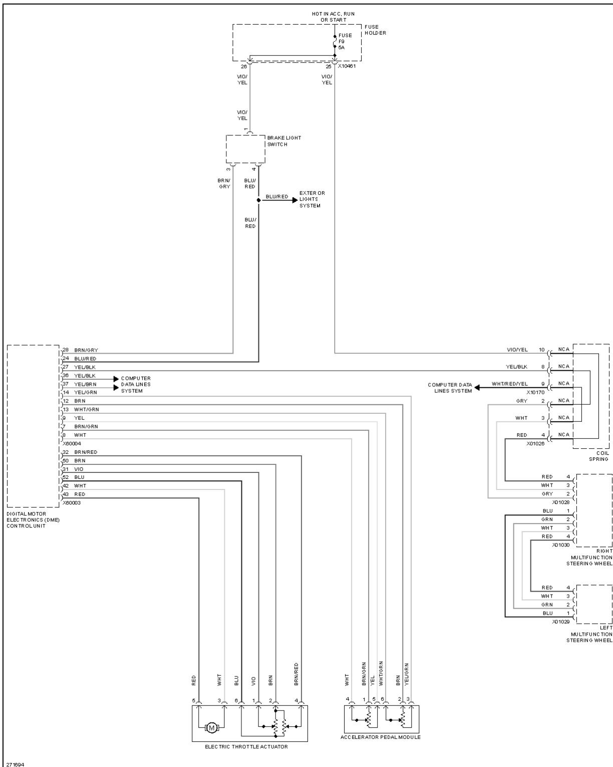
**Fig. 23: 4.4L, Cruise Control Circuit**
