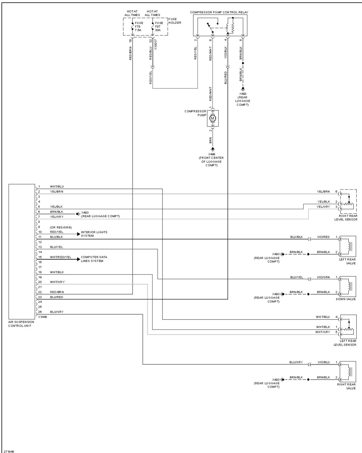
**Fig. 28: Electronic Suspension Circuit, W/ Single Axe**
