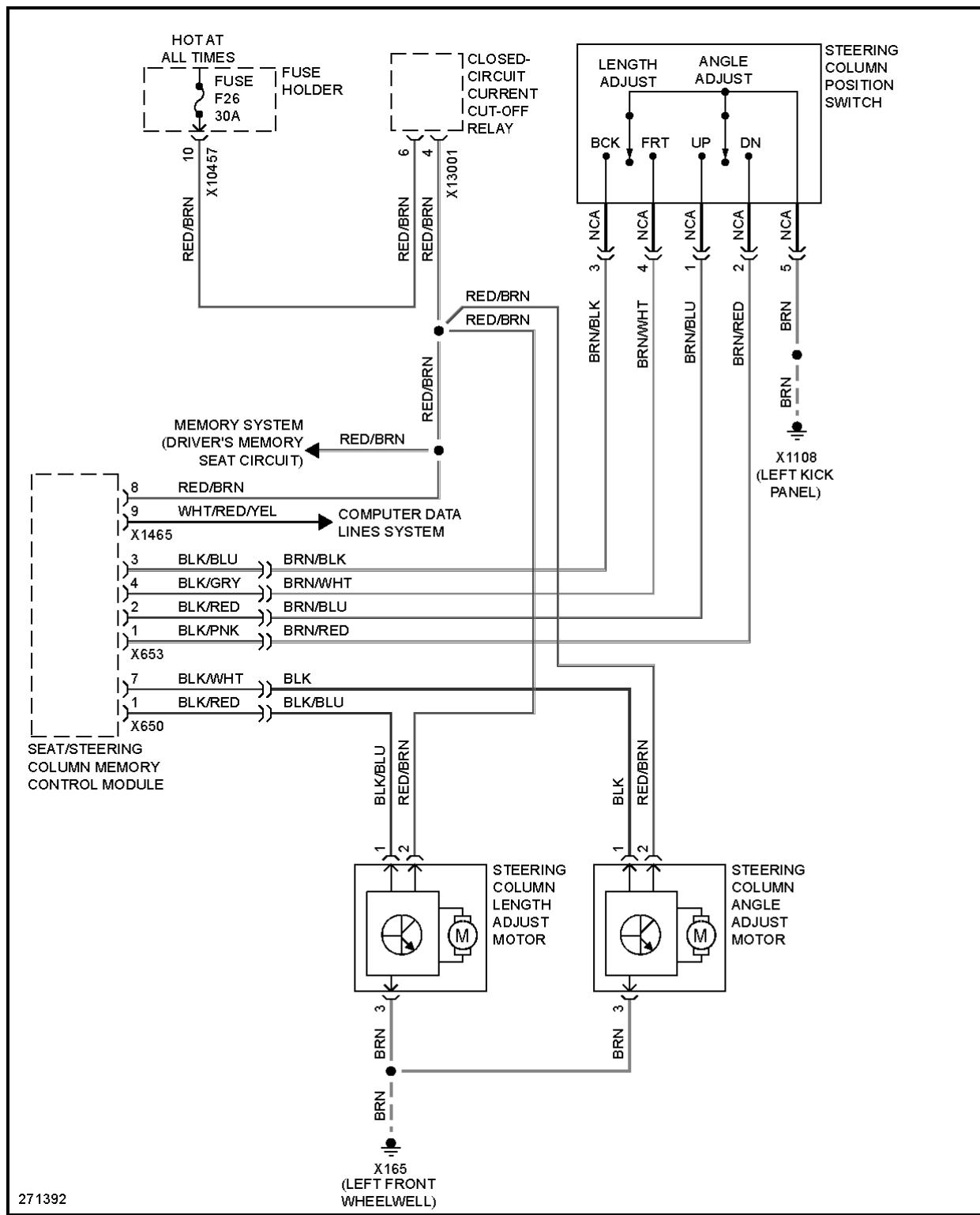
**Fig. 74: Steering Column Memory Circuit**
