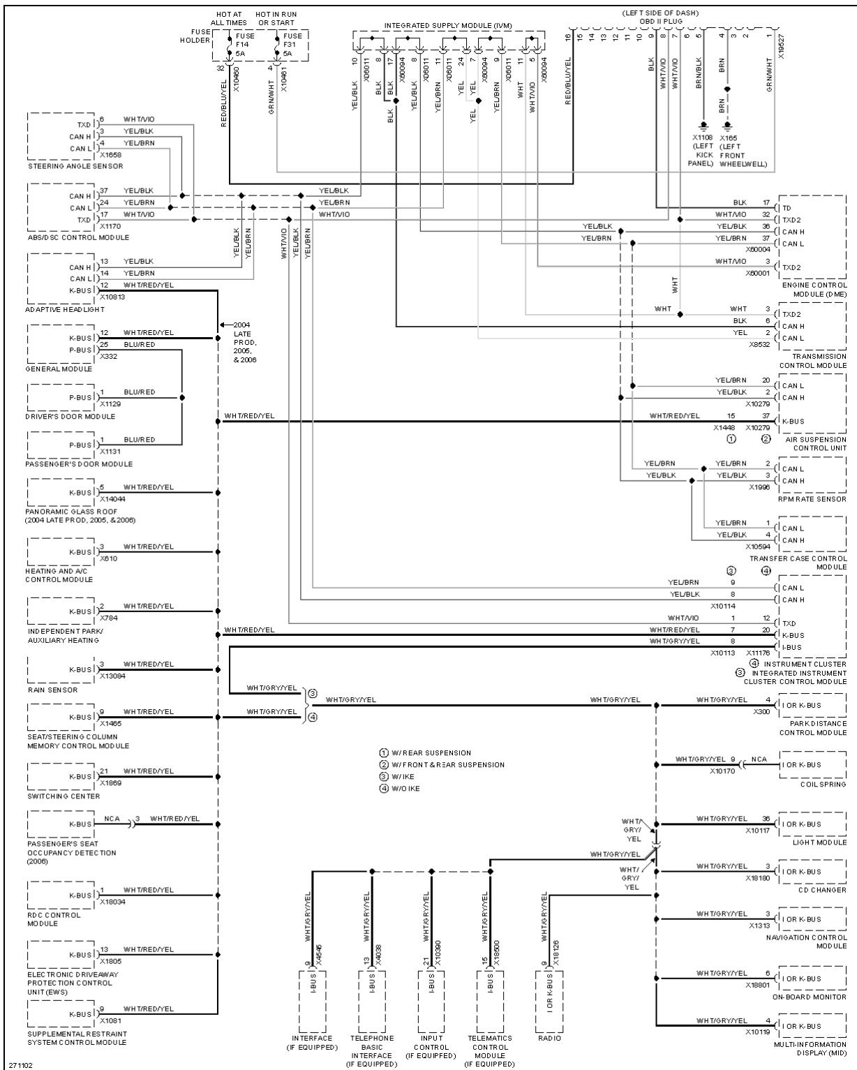
**Fig. 17: 4.4L, Computer Data Lines Circuit**
