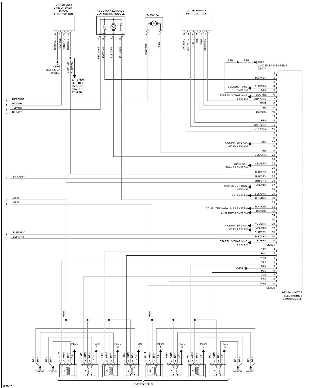
**Fig. 38: 4.4L, Engine Performance Circuit (6 of 6)**
