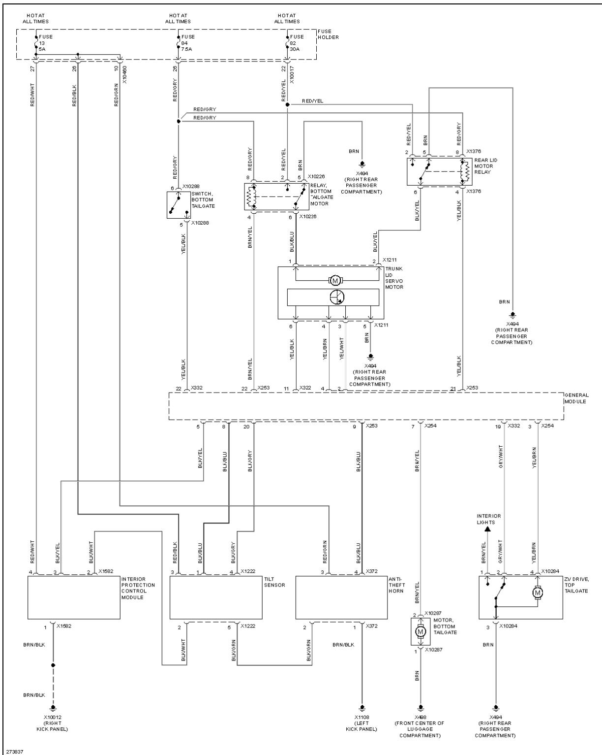
**Fig. 11: Anti-theft & Central Locking Circuit (3 of 3)**
