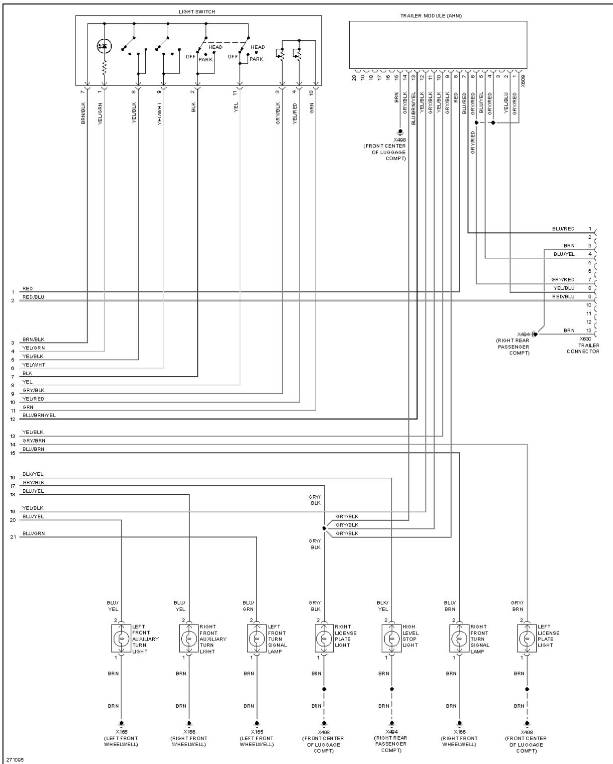
**Fig. 47: Exterior Lamps Circuit (2 of 2)**
