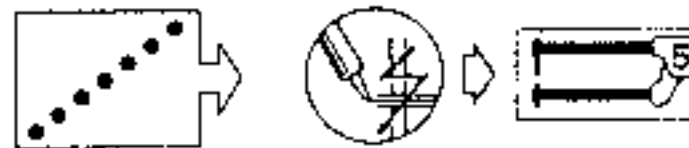
(A) 7 spots through 3 thicknesses
