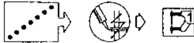
(A) 2 spots through 3 thicknesses
