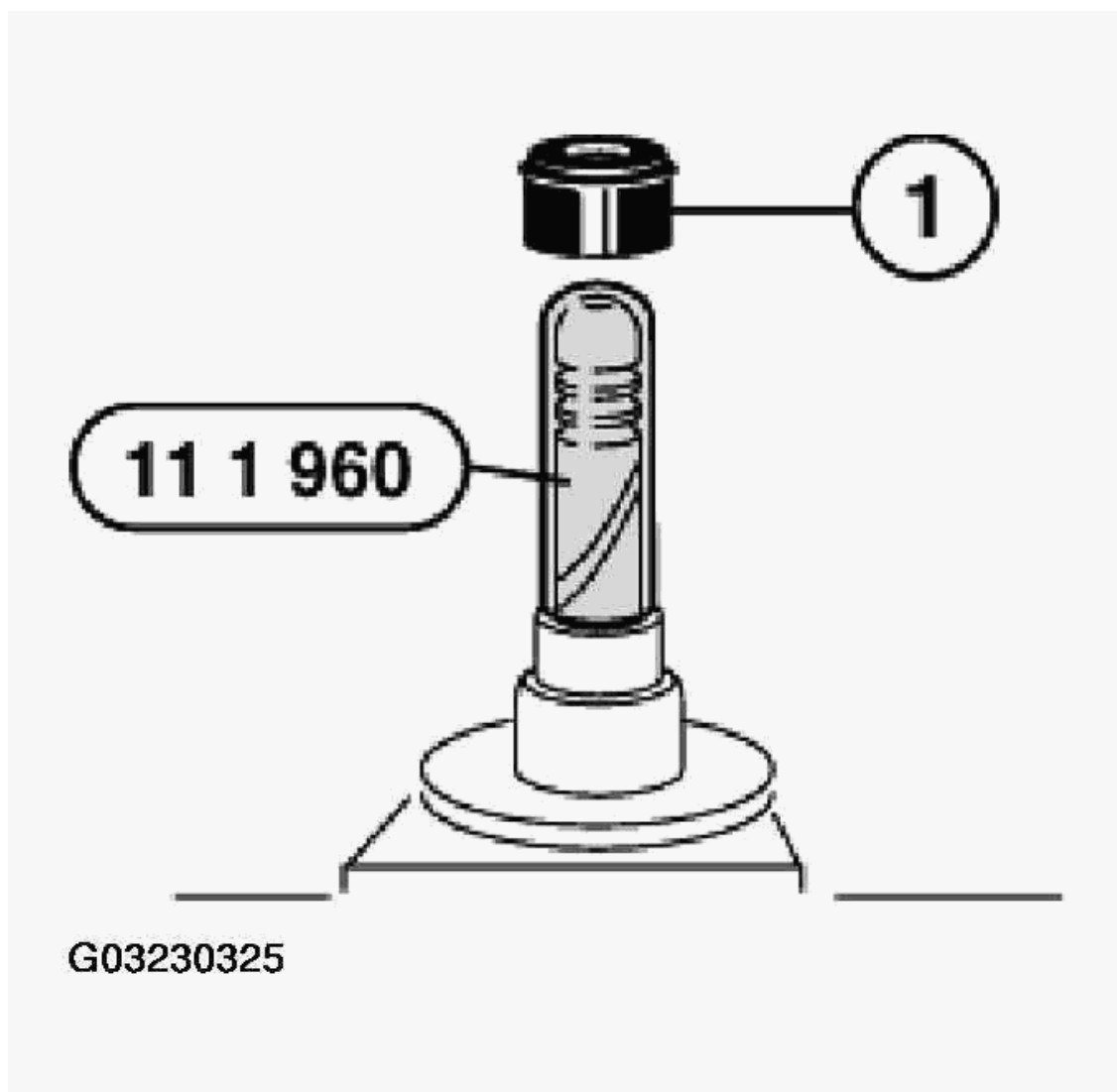
Fig. 283: Installing Valve Stem Seal On Assembly Sleeve Courtesy of BMW OF NORTH AMERICA, INC.
