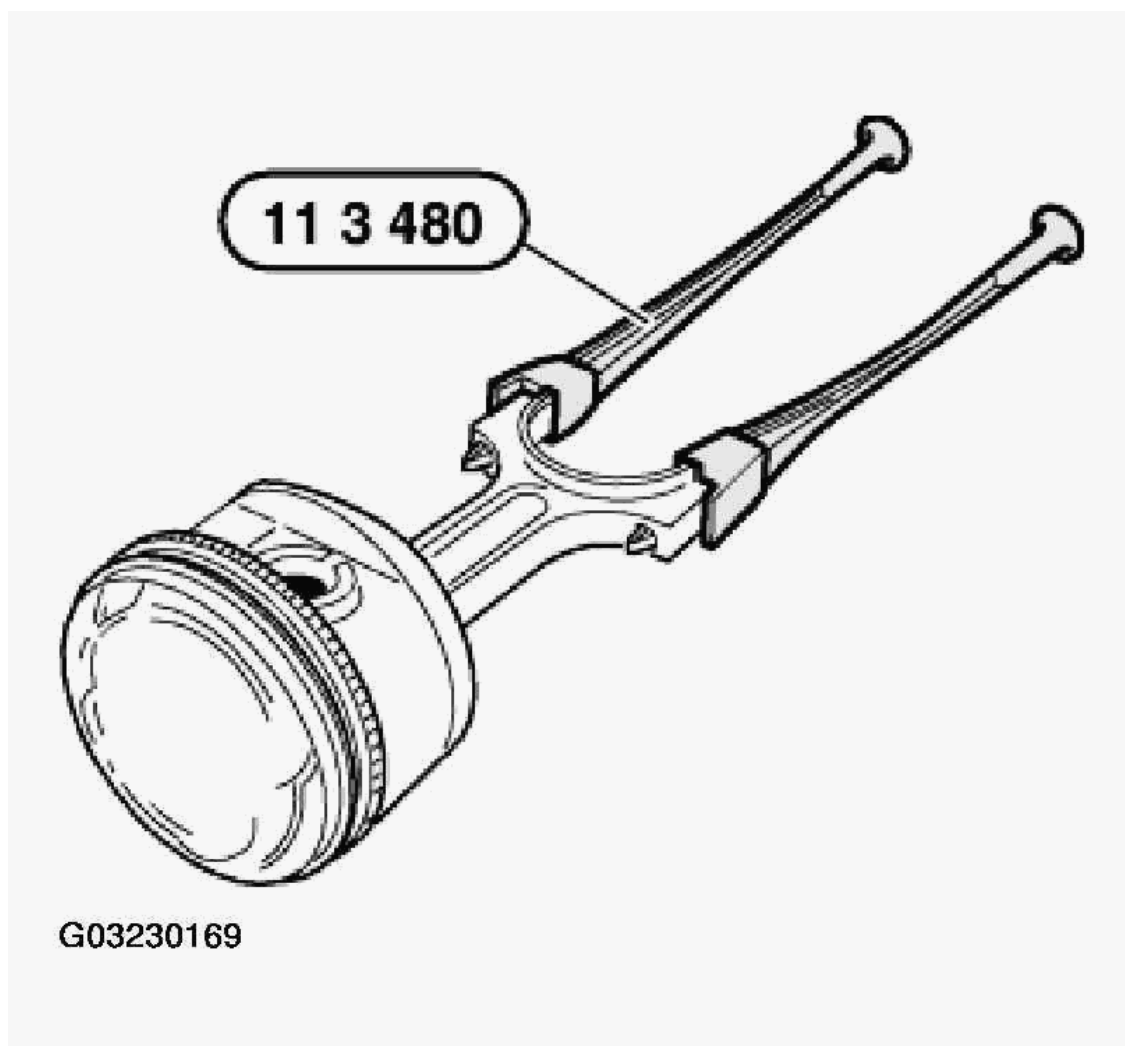
Fig. 129: Identifying Conrod With Piston Courtesy of BMW OF NORTH AMERICA, INC.
