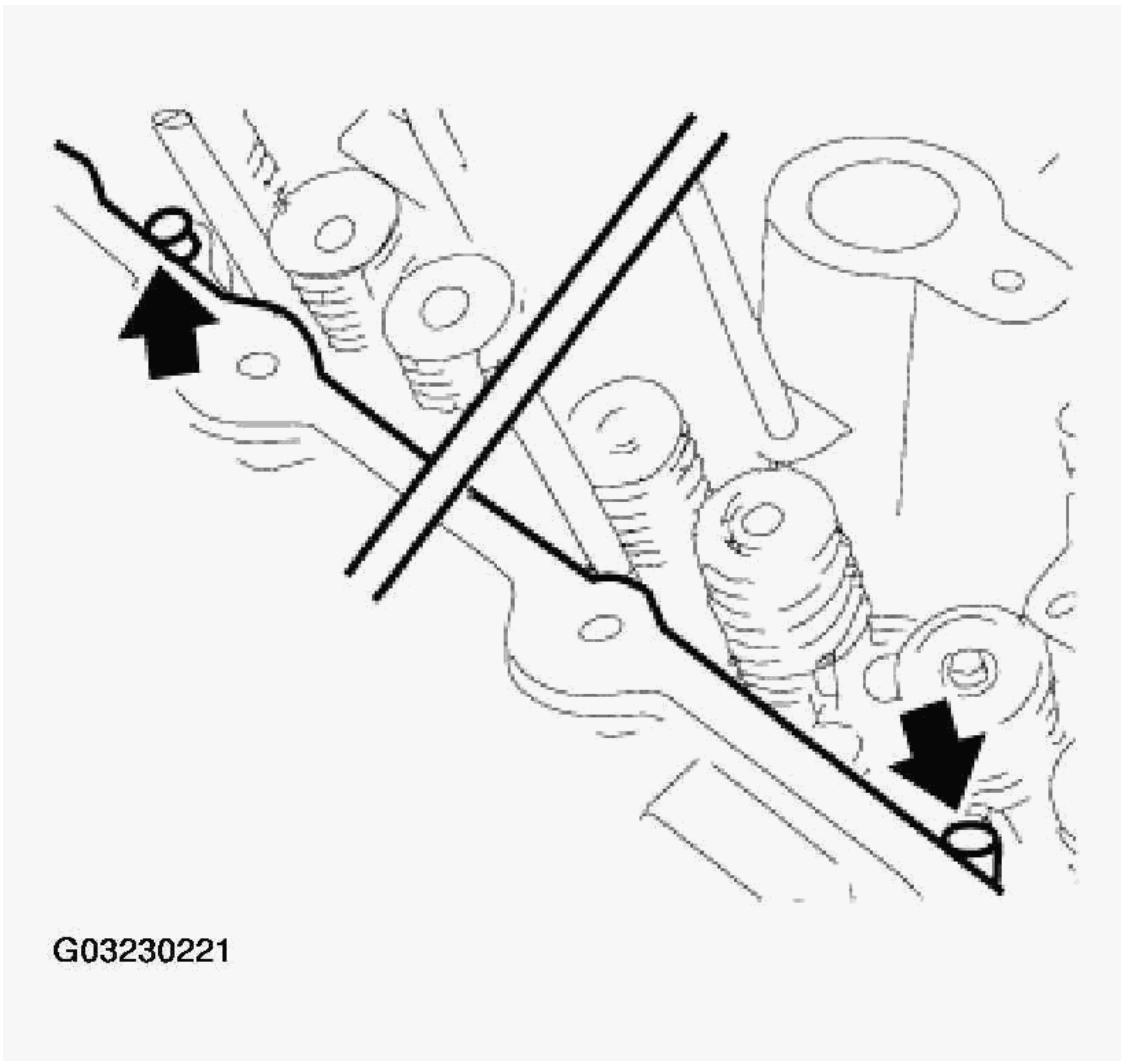
Fig. 179: Installing Bearing Strips Courtesy of BMW OF NORTH AMERICA, INC.
