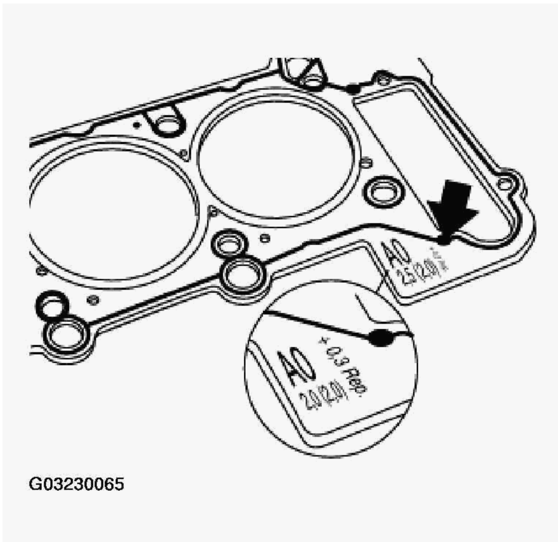
Fig. 39: Locating Repair Cylinder Head Seal Courtesy of BMW OF NORTH AMERICA, INC.
