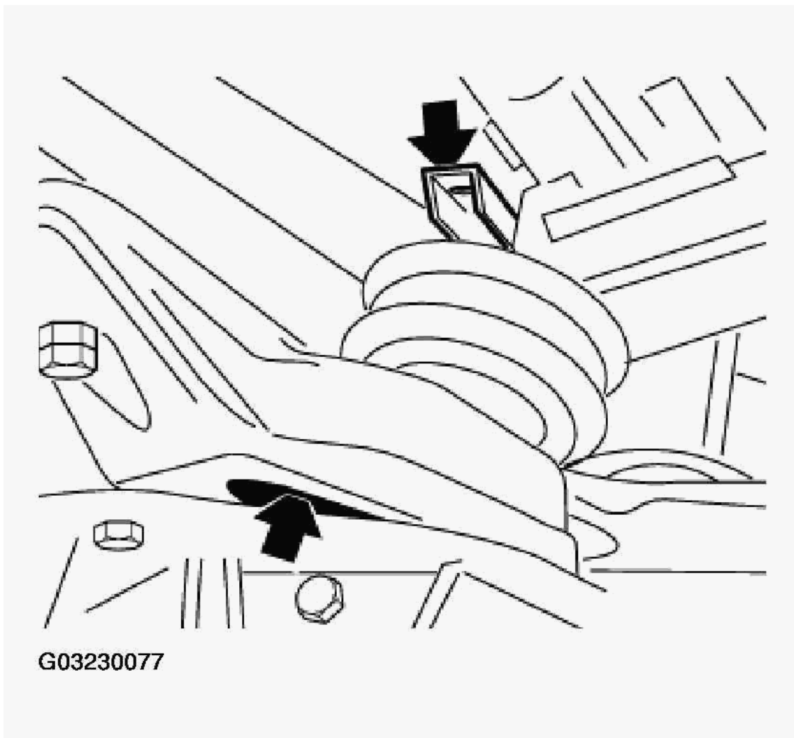
Fig. 51: Locating Top/Bottom Of Left/Right Engine Mounts Courtesy of BMW OF NORTH AMERICA, INC.
