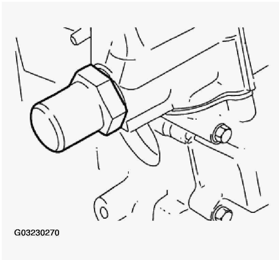
Fig. 228: Removing Cylinder For Chain Tensioning Piston Courtesy of BMW OF NORTH AMERICA, INC.
