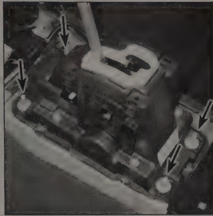
3.10 To remove the shifter assembly, remove the four mounting nuts
