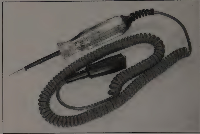
2.5b A test light is a very handy tool for checking voltage
