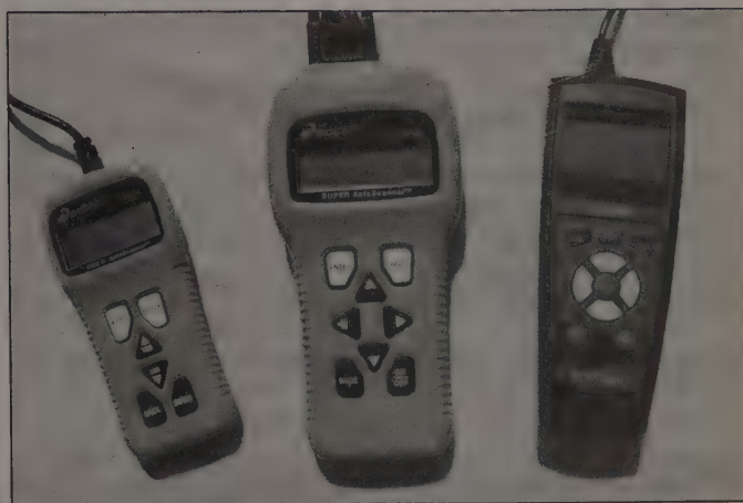
2.4b Hand-held scan tools like these can extract computer codes and also perform diagnostics
