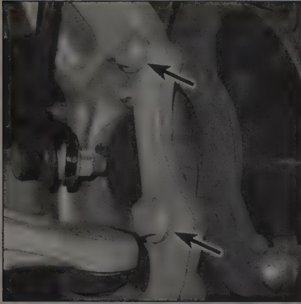
6.6a Caliper mounting bracket-to-knuckle bolts (typical front caliper shown, rear caliper similar)
