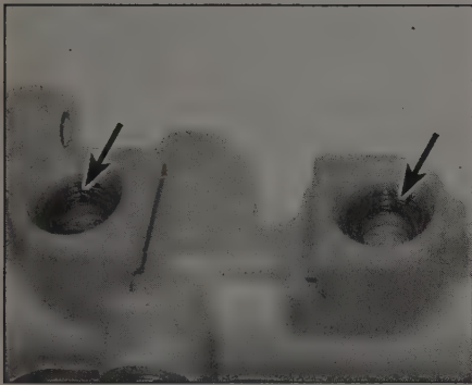
7.7 After the reservoir has been removed, replace the O-rings with new ones
