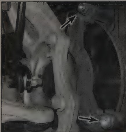
4.6h Remove the two caliper guide pins
