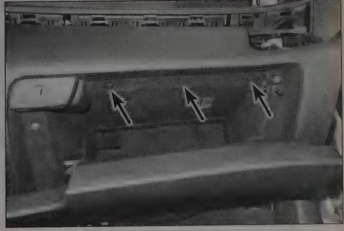
24.38 Remove the mounting fasteners from inside the glove box
