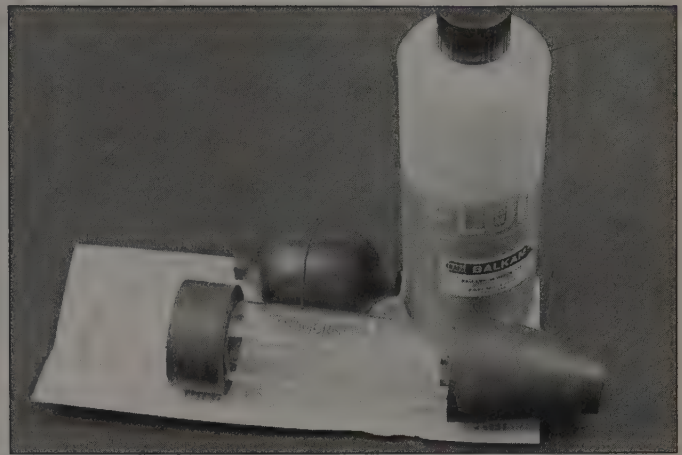
2.5a The combustion leak detector consists of a bulb, syringe and test fluid
