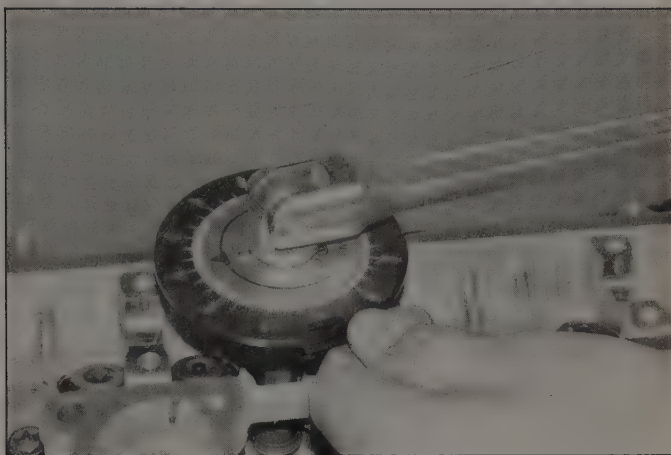
12.28b You can use a torque angle gauge, or you can carefully note the starting and stopping points of the wrench handle
