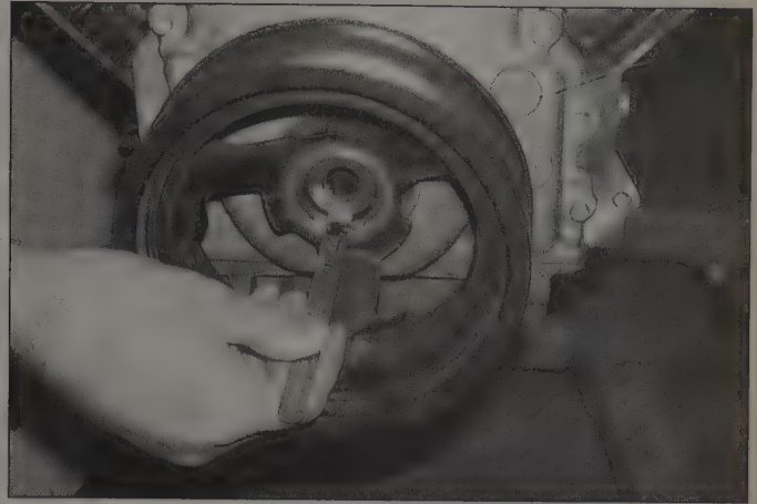
10.5b Before the new crankshaft bolt is installed and tightened, the balancer must be measured for proper depth - it should match the original measurement taken before removal
