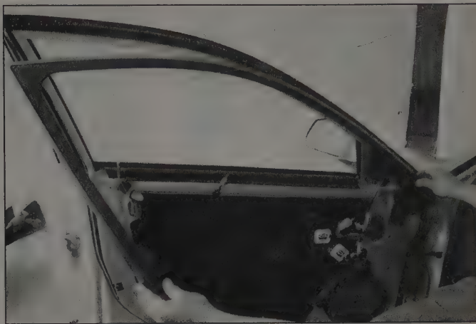
13.15 Disengage the window frame trim panel
