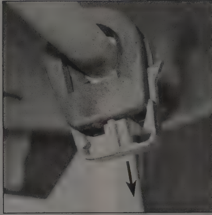
9.18b To disconnect the quick disconnect lines, pull out the lock . . .
