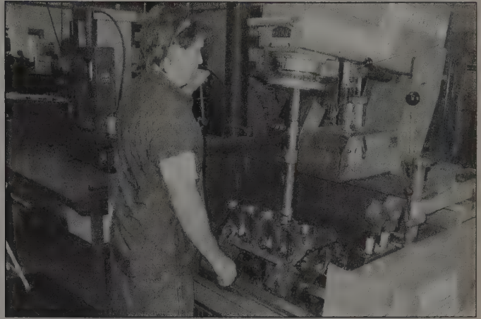
1.2 If the cylinders are bored, the machine shop will normally hone the engine on a machine like this
