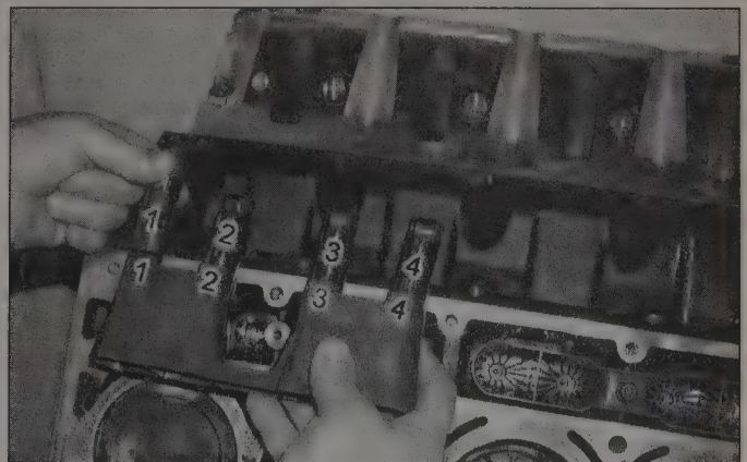
13.2b Once the lifters and retainers are removed from the block they can be marked (for location and installation purposes) and inspected
