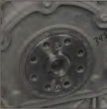
18.7 Alignment dowels installed to the rear main oil seal housing bolt holes
