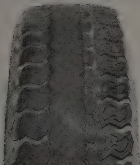
INCORRECT TOE-IN OR EXTREME CAMBER
