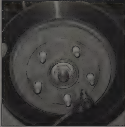
6.6b A screw secures the disc to the hub (rear disc shown, front disc identical)
