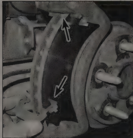
4.6f Remove the brake pad support plates from the caliper bracket
