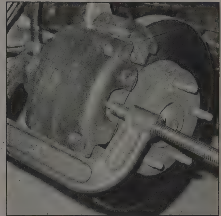
4.6a Depress the piston into the bottom of its bore in the caliper with large C-clamp to make room for the new pads - make sure the fluid in the master cylinder reservoir doesn't overflow
