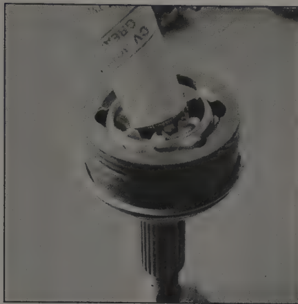
10.12a Pack the outer CV joint assembly with CV grease . . .
