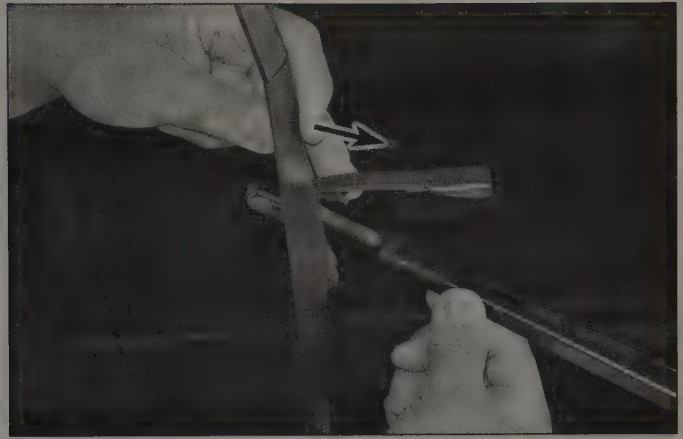
8.4b . . . and pull the wiper blade in the direction of the arrow to separate it from the arm
