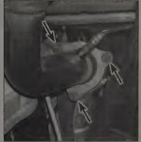
8.4 Remove the exhaust pipe-to-manifold nuts
