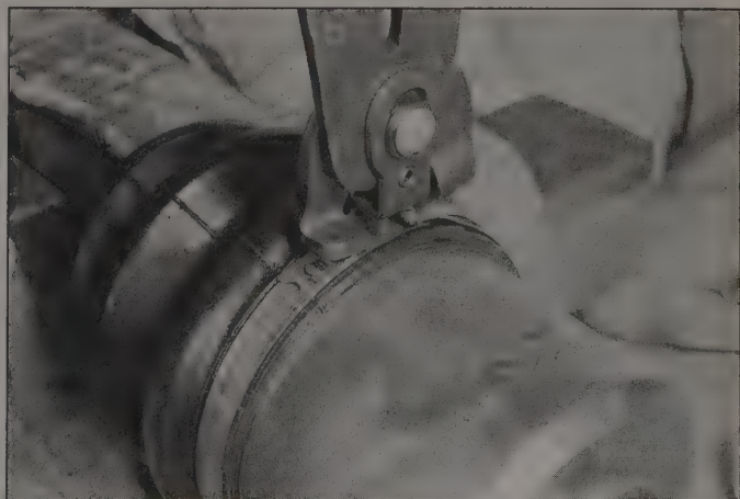
10.15 To install crimp-type boot clamps, you'll need a pair of special crimping pliers (available at most auto parts stores)
