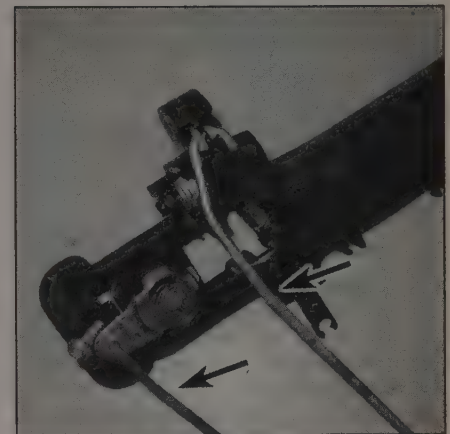
15.22 To disconnect the actuator rods from the outside door handle reinforcement, angle the reinforcement as necessary to disengage each rod
