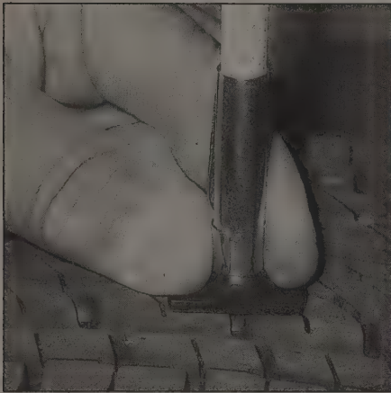
5.2 A tire tread depth indicator should be used to monitor tire wear - they are available at auto parts stores and service stations and cost very little
