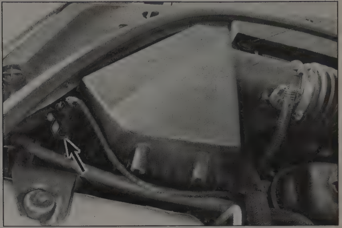
12.1 The BARO sensor is located on the air filter housing cover (3.0L V6 engine)
