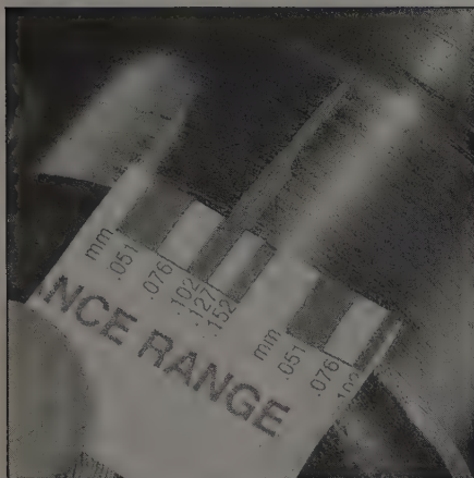
10.21 Use the scale on the Plastigage package to determine the bearing oil clearance - be sure to measure the widest part of the Plastigage and use the correct scale; it comes with both standard and metric scales
