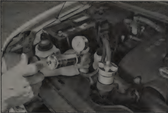
2.2 The cooling system pressure tester is connected in place of the pressure cap, then pumped up to pressurize the system
