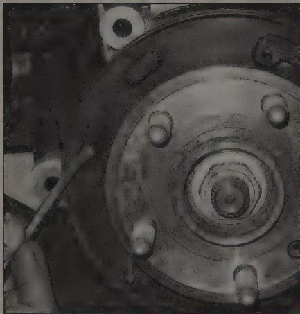
12.4h Clean the backing plate with brake cleaner and lightly lube the shoe contact points with brake grease
