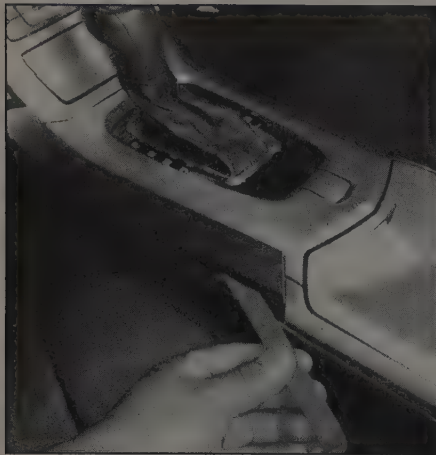
23.7 Pry out the outer trim panels from the center console
