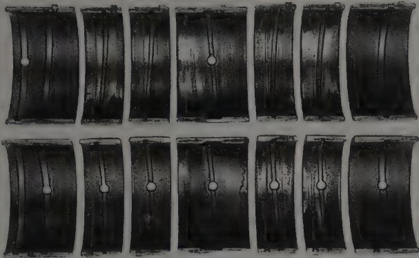
A warped crankshaft caused this pattern of severe wear in the center, diminishing toward the ends
