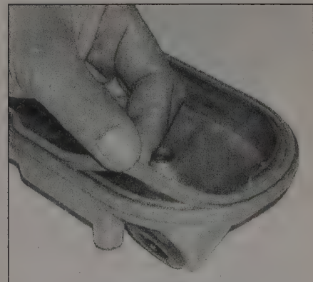
4.12 Position the new gasket in the valve cover lip
