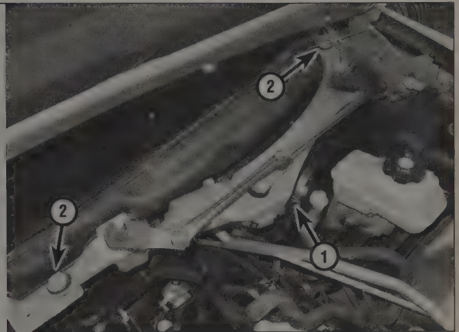
18.3 Wiper motor electrical connector (1) and assembly mounting bolts (2)
