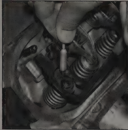
6.8 Once the spring is depressed, the keepers can be removed with a small magnet or needle-nose pliers (a magnet is preferred to prevent dropping the keepers)
