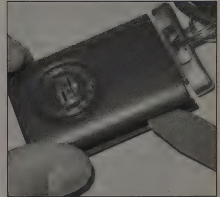
24.14 Using a coin, carefully pry the halves of the transmitter apart
