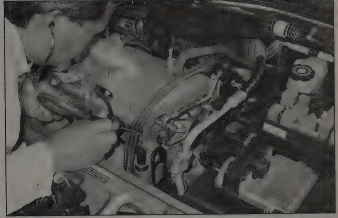
2.9 An automotive stethoscope is used to listen to the fuel injectors in operation
