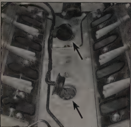
9.10 5.7L V8 engine knock sensor locations
