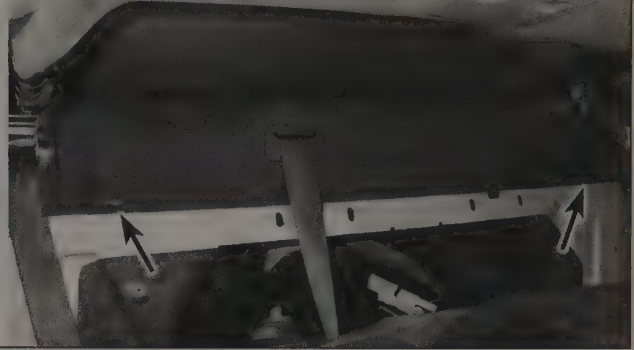
28.13 Remove the plastic push pins from the front of the package tray panel
