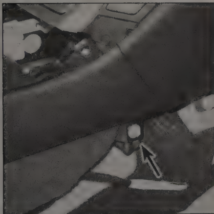
23.12 Pull down the carpet and remove the console front lower fasteners
