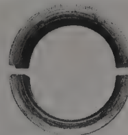
Damage from excessive thrust or insufficient axial clearance
