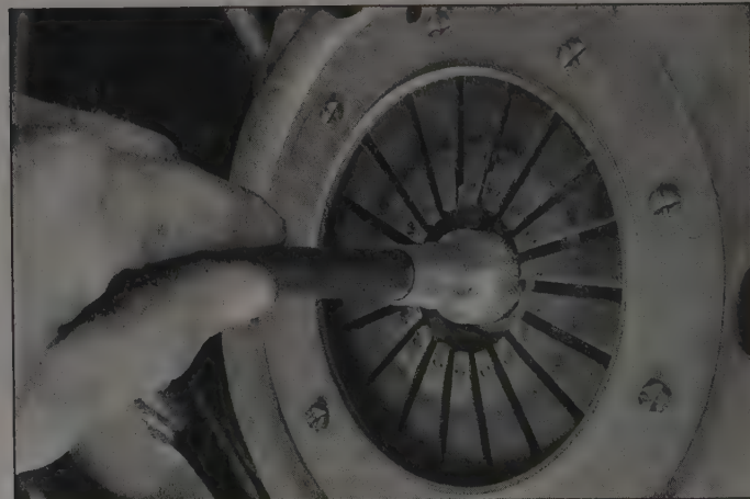
6.16 Center the clutch disc in the pressure plate with a clutch alignment tool
