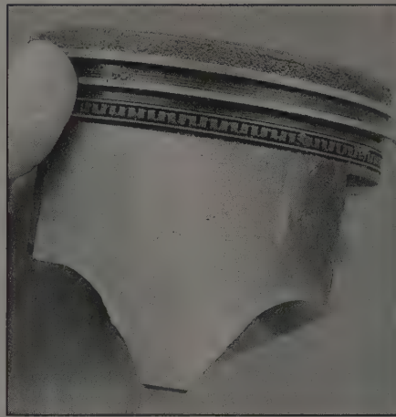
1.6 Uneven piston wear like this indicates a bent connecting rod
