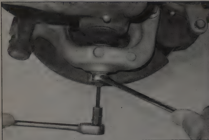
5.5 Using hand tools only, hold the ballstud with an Allen wrench and loosen the ballstud nut with a wrench
