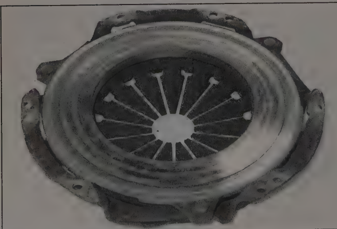
6.11b Inspect the pressure plate surface for excessive score marks, cracks and signs of overheating
