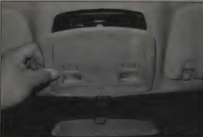
17.44 To remove an overhead panel, carefully pry it off with a trim removal tool or screwdriver
