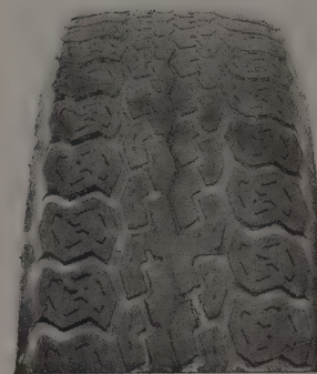
FEATHERING DUE TO MISALIGNMENT
