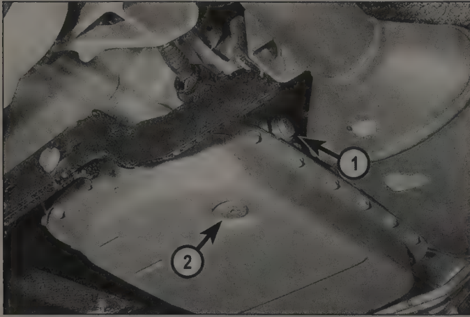
7.4 Location of the five-speed automatic transmission fluid check plug (1) and the drain plug (2) (2007 and earlier models)
