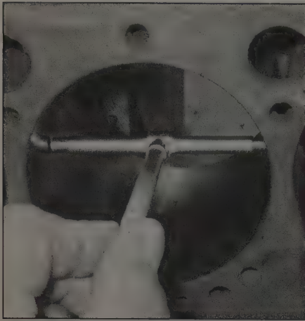
1.5 A bore gauge being used to check the main bearing bore
