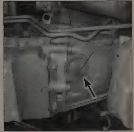
5.21a Remove the torque converter cover plug . . .
