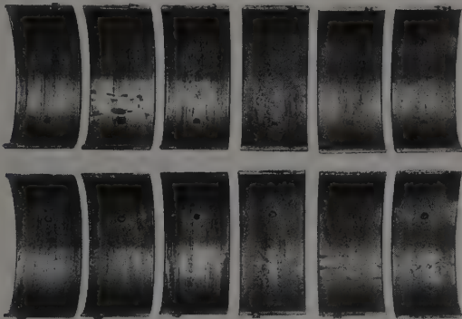
Result of dry start: The bearings on the left, farthest from the oil pump, show more damage
