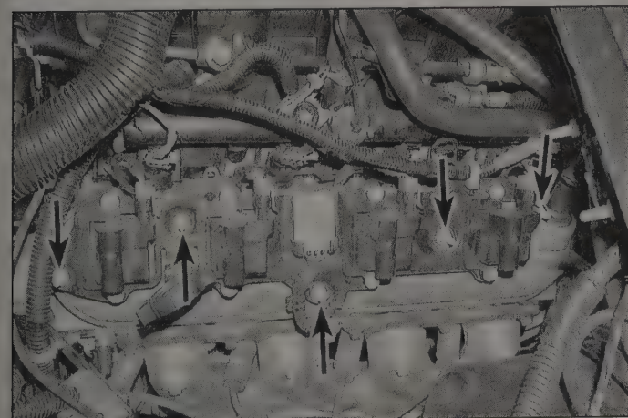
6.8 Remove the ignition coil bracket bolts (5.7L V8 engine shown, other V8 engines similar)
