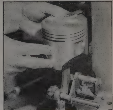
1.4 A machinist checks for a bent connecting rod, using specialized equipment
