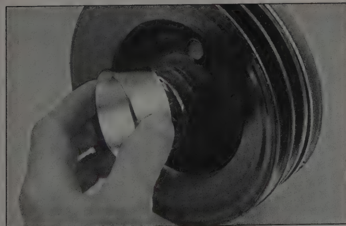
11.5 If the sealing surface of the pulley hub has a wear groove from contact with the seal, repair sleeves are available at most auto parts stores
