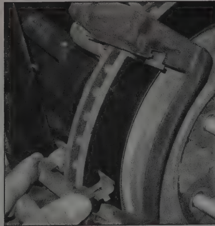
4.7e Remove the brake pad support plates from the caliper bracket, then remove the remaining caliper bolt and secure the caliper to the suspension with a length of wire
