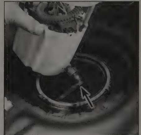
7.5 Lift the module out at an angle and disconnect the transfer tube
