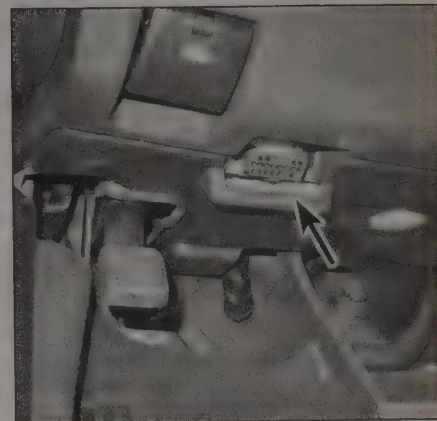
3.1 The Data Link Connector (DLC) is located at the lower edge of the dash, below the steering column
