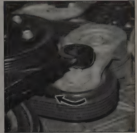
24.5 To remove the drivebelt, insert a 1/2-inch drive ratchet or breaker bar into the square hole and rotate the tensioner arm to relieve belt tension - V6 model shown, other models similar
